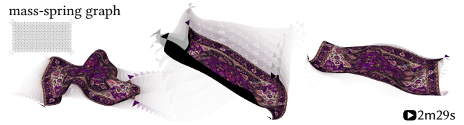
Fig. 14. A carpet springs to life with complementary dynamics provided by a mass-spring cloth simulation [Baraff and Witkin 1998]. Our constraints augment the local-global solver of Liu et al. [2013].
