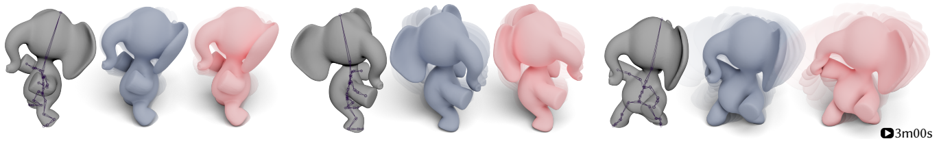
Fig. 16. A motion capture sequence controls the skeleton rigged inside of an elephant. The trunk and ears are not articulated by the skeleton so freely receive lively secondary effects. The material parameter (i.e., Young's modulus) of the blue elephant is set to be stiffer than the pink elephant.
